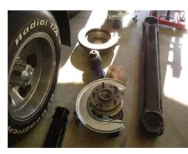
The lower shock absorber mount forging goes in from the front through the ears and the strut rod, and the flat on the end of the forging mates up with the flat on the rear ear. The splash
